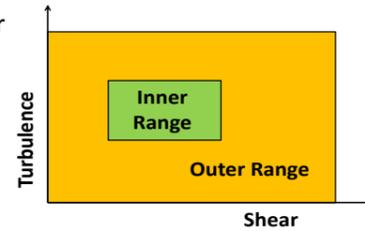
• **Outer range conditions are relatively frequent** and therefore the calculation of turbine power output in outer range conditions is an important consideration in wind energy resource assessment.
